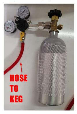
The last connections are the to the KEG COUPLER which is connected to the KEG. The hose coming from the Co2 gas cylinder and the KEG TAP are connected to the coupler as seen below.
