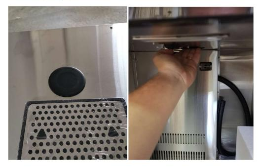
The KEGORATOR TAP and hose can pass through. The TAP can then be fastened using the washer and nut assembly on the bottom of the TAP as seen below. The Hose will have to be connected to the KEG.
