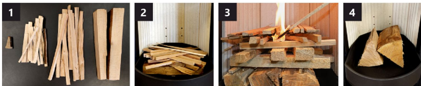
Fig. 1 Wood preparation procedure in the combustion chamber
