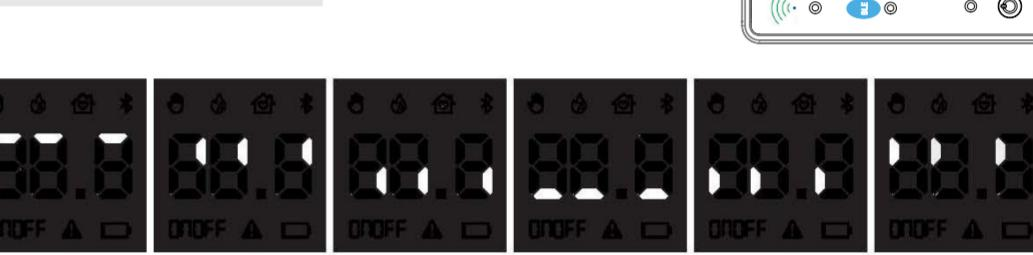
In the case of a non-paired remote control, a circular digit lighting sequence will be displayed at each start-up (for battery insertion or awakening by pressing a button).
