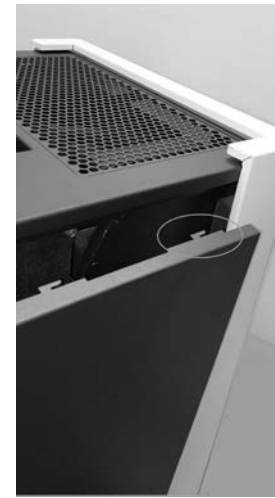
Fig. 23 - Extraiga la pared lateral
