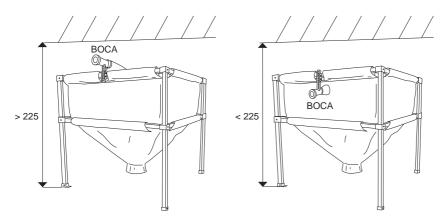
Once the final position of the silo has been decided, make sure that it is positioned with a spirit level and then fix the base (INFSP) to the floor with the dowels and screws provided.
