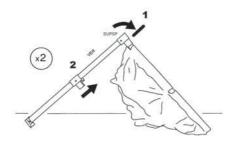
Raise the silo from the other side and insert the two remaining vertical tubes (VER).
