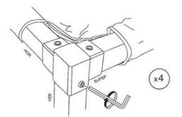
Insert the intermediate tubes (HOR) into the intermediate fittings (INTSP) and tighten the screws. Make sure that all the eyelets are equally stretched upwards.
