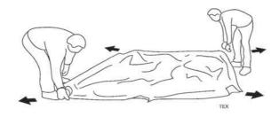
Insert the horizontal tubes (HOR) into the four upper fabric eyelets (TEX).
