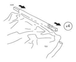
Insert the horizontal tubes (HOR) into the upper fittings (SUPSP) and tighten the screws.
