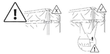
Before filling the tank with a tanker, check that the inlet tube is fully inserted and, in any case, beyond the seam of the fabric inlet.
