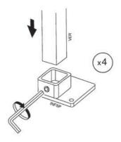
Insert the intermediate fittings (INTSP) into the vertical tubes (VER) fixing them to the height specified in the table and tighten the screws.
