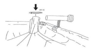
Insert the filling inlet until it exceeds the seam of the fabric inlet and then tighten the clamp. It is recommended an adequate grounding at the filling inlet.
