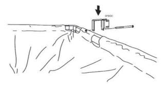
Fix the filling inlet (BOCA) with the storz attachment which must be inclined about 10/15 ° downwards. If there is no space above the silo, rotate the fixing bracket (SPBOC) 180 ° and install the filling inlet using the lower inlet. In this case the capacity of the silo will be slightly reduced (see model specifications).
