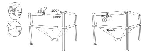
Insert the small clamp (ABR100) into the upper filling inlet of the silo.
