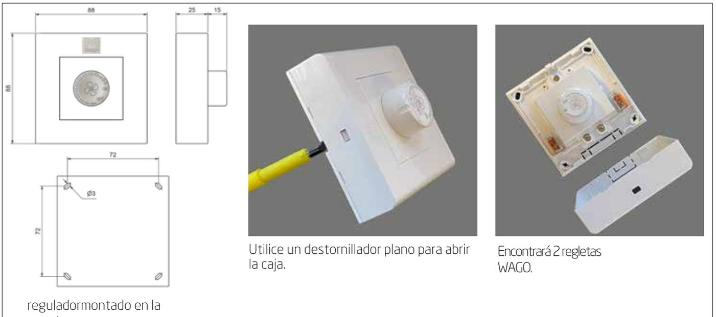
The technical drawings show the dimensions of the regulator box: 88mm width and height, 25mm depth, and 15mm for the side flange. The front panel has a 72mm square cutout with a 53mm diameter hole. The photos show the box being opened with a flat screwdriver and the internal WAGO terminals.
