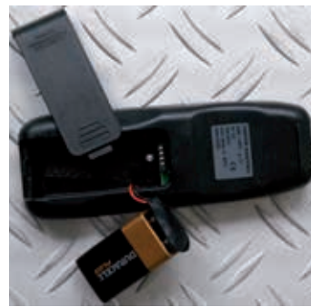
Replacing the batteries in the remote control
