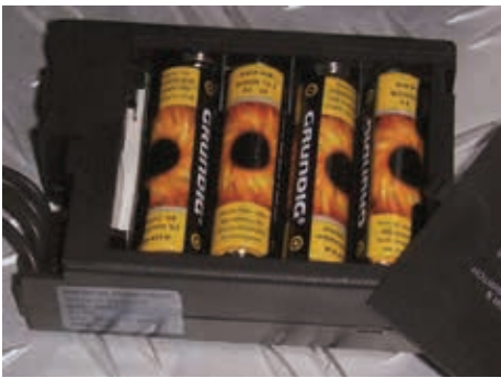
Replacing the batteries of the receiver
