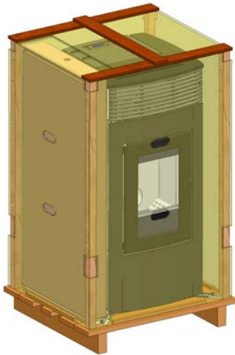
STOVE PACKAGING WITH METAL CLADDING
