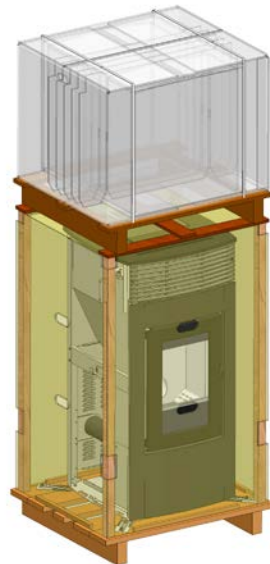
STOVE PACKAGING WITH CERAMIC CLADDING (ABOVE)
